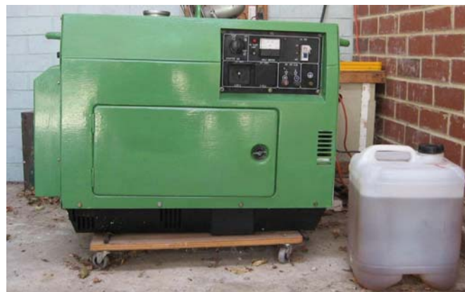
5 kW Diesel generator running on biodiesel
